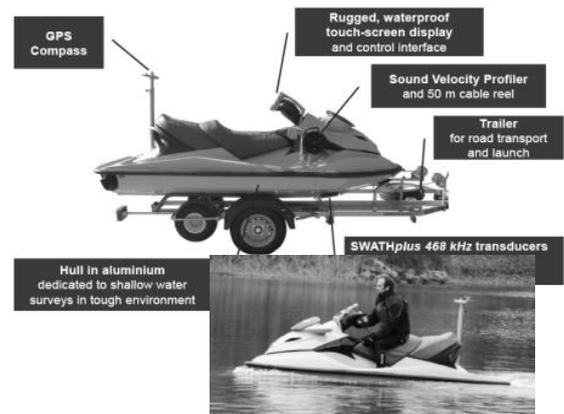
**Gambar 8.** Sistem Jet ski Batimetri
